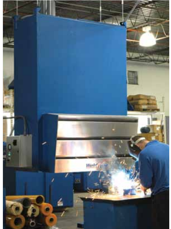
RoboVent WeldPro for a Manual Process.
