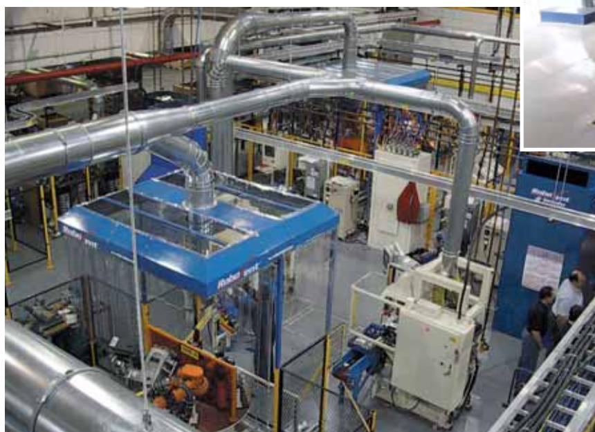
RoboVent Resistance Welding Air Cleaning System ducted to each station
