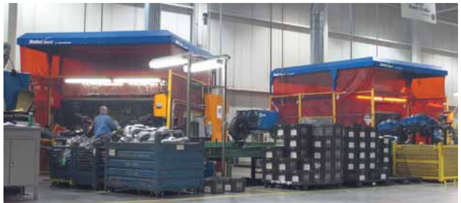
RoboVent FlexMount System for Robotic Welding.
