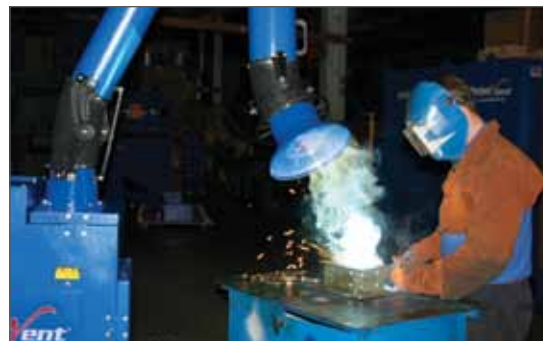
RoboVent Trans4mer with 8" articulated fume arm.
