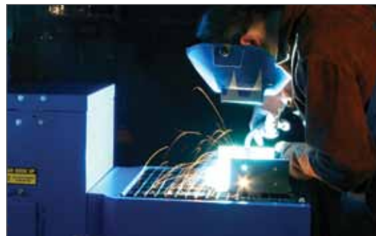
RoboVent Trans4mer with optional downdraft collector.
