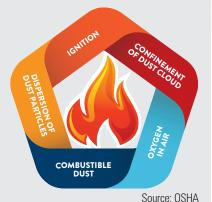
If the quantity of dust in suspension in the air that is moving through a dust collection system is above what is called the minimum explosive concentration (MEC), then the suspension can potentially explode in the presence of an ignition source (e.g., a welding gun).
