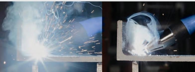
This norm is, in practice, exceeded in many workplaces. To comply, companies may adopt various measures including room ventilation, mobile extraction hoods, or personal protective equipment such as dust masks or ventilated helmets. The effect of these is often insufficient:
